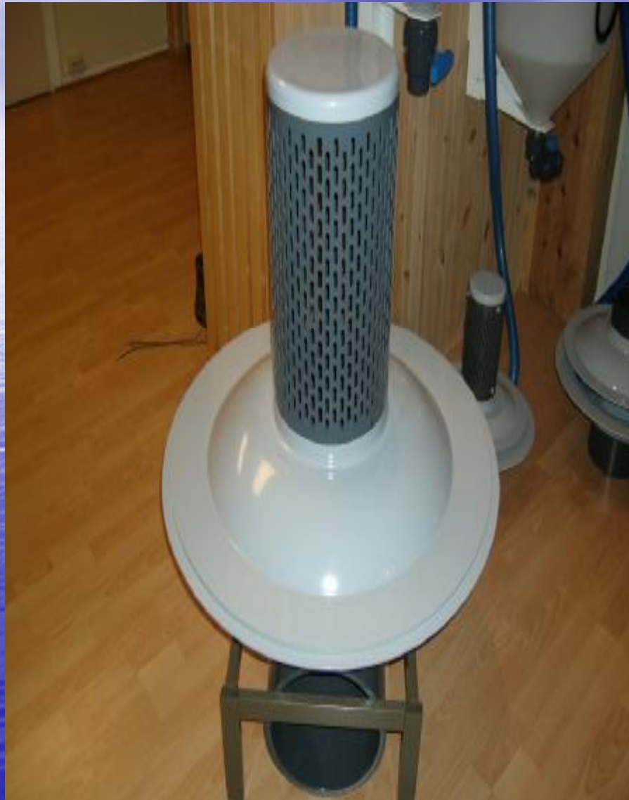
Figure 2. The ECO-TRAP™ particle trap is an advanced double drain design that concentrates much of the settleable solids in only 5 percent of the water flow leaving the fish culture tank (B). (after Hobbs et al., 1997). (ECO-TRAP is a trademark of AquaOptima AS, Pir Senteret, 7005 Trondheim, Norway, U.S. Patent No. 5,636,595.)
